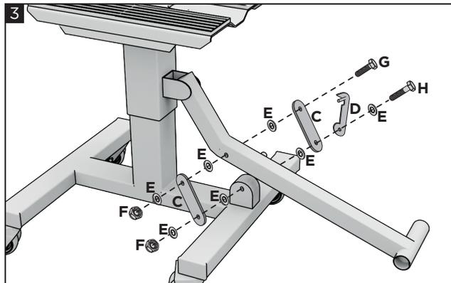
**Fix the brackets (C) and the safety (D) using the screw (G), the screw (H), the washers (E) and the nuts (F). Tighten the screws taking care that the lever (D) does not be blocked.**
