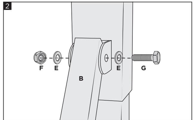
**Fix the lever using the screw (G), the washers (E) and the nut (F) as shown in the figure. Tighten the screws taking care that the lever (B) does not be blocked.**
