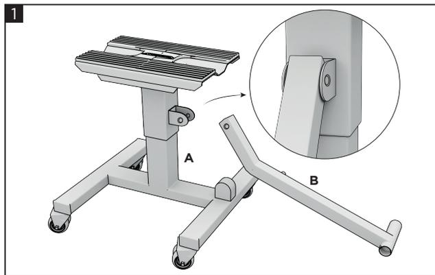
**Position the lever (B) in the appropriate seat on the stand (A) matching the holes.**
