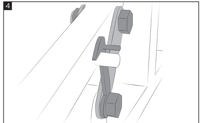
**Tighten the screws without preventing the movement of the parts, checking that everything works properly.**
